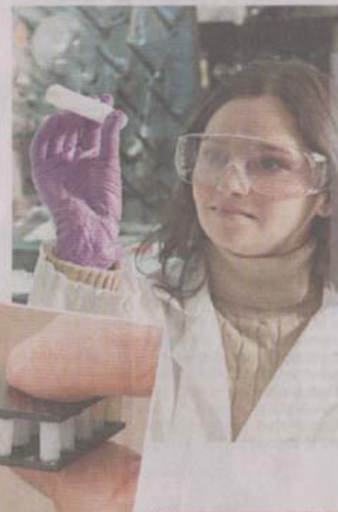
A researcher examines a tubular Aerogel material sample in its "green" state.
